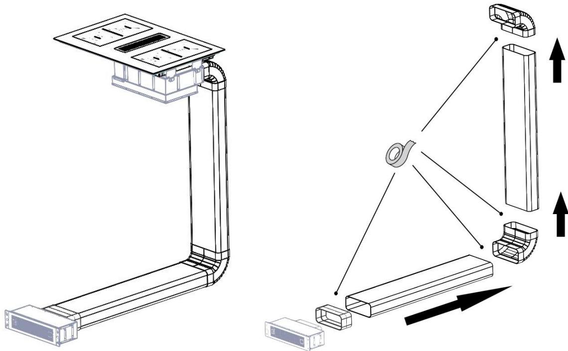
**Connect the air duct components to each other and insert them into the outlet connection at the back of the cooktop.**
