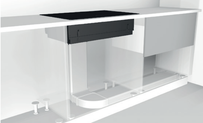
Installation example with exterior exit
