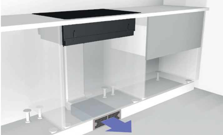
Installation example with socle grid (90376)
